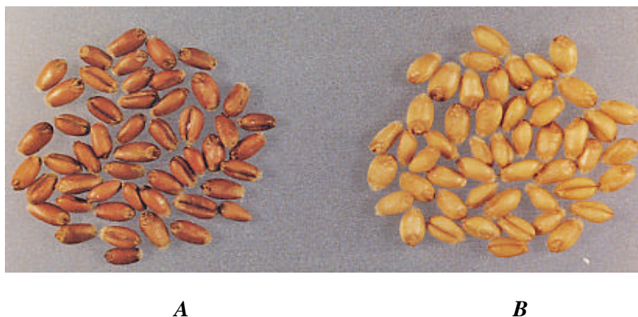
Fig. 5. Sodium hydroxide (NaOH) test: (A) Red wheat, and (B) white wheat.
