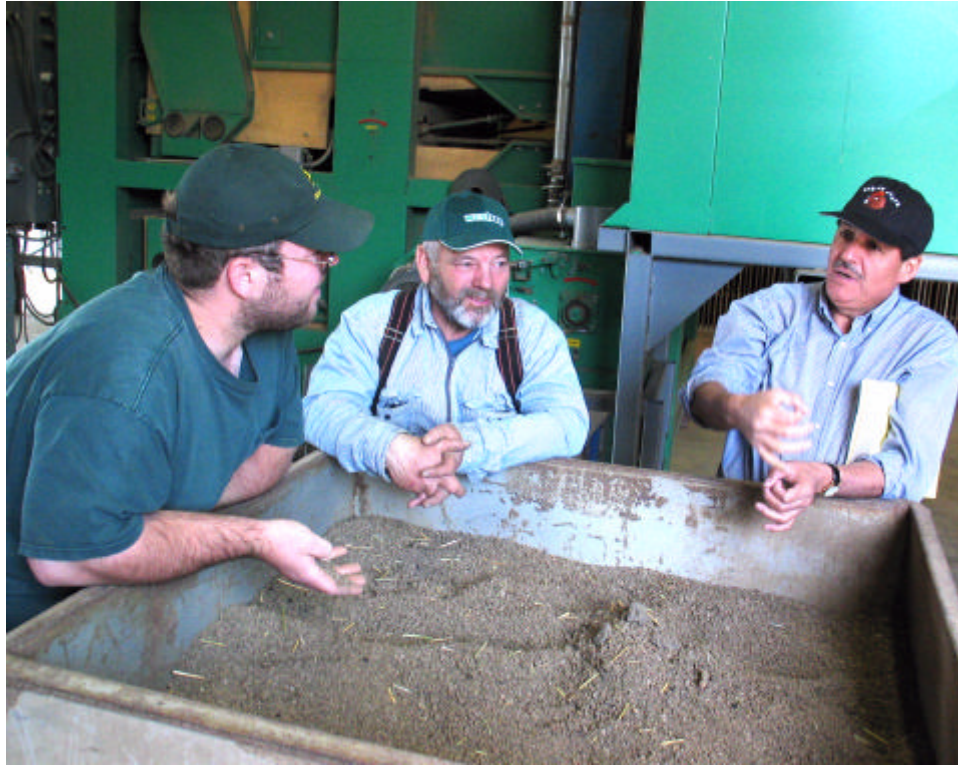
Khalen Boyer, Bill Boyer and Adriel Garay observing a bin full of soil that was separated by an aspirator before feeding the seed into the air-screen machine
