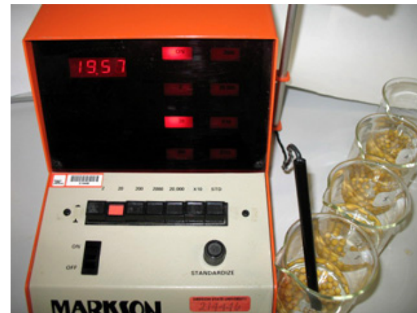
Electric Conductivity Test in soybean. High quality seeds have lower electric conductivity readings than low quality seeds.
